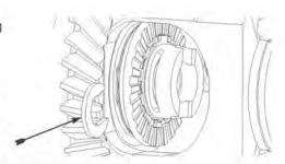
**18.** Rotate ring gear side wheel 1/4 turn back so that the spacer paddle and the opening in the synchro ring is facing out towards you.
