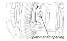
37. Feel through pinion shaft opening and verify both spacers and drivers are fully seated onto couplers. Verify all 8 saddle springs are fully seated in holes.
