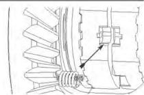
Visually inspect notches in spring slot to make sure inner spring is fully seated.
