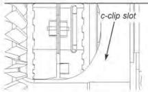
34. Making sure drivers stay engaged with couplers, carefully rotate wheels until c-clip slot is accessible. Verify c-clip groove on axle is accessible through c-clip slots on driver and spacer.
