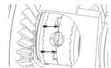
**25.** Wedge both drivers in engagement with couplers. Rotate driver's side wheel forward 1/4 turn to reveal spring slot.
