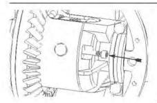
**40.** Insert retaining bolt/roll-pin into case/shaft. Tighten retaining bolt firmly.
