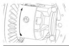
**38.** Keeping couplers and drivers stationary, rotate case 1/4 turn forward to align pinion shaft opening with driver saddles.
