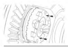
**20.** Press driver down onto coupler. Driver teeth should be fully engaged all the way around.
