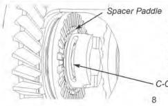
**16.** Place an active spacer onto the ring gear side coupler as shown. Make sure spacer paddle is seated in the paddle opening of the synchroring and c-clip slot is facing out towards you.
