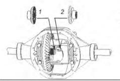
**14.** Install couplers inside differential case, ring gear side first.
