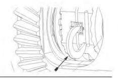
36. Making sure drivers stay engaged with couplers, carefully rotate both wheels backwards 1/4 turn to expose pinion shaft opening.
