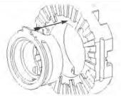
21. Insert the second active spacer into the slotted driver. Seat the spacer paddle at the paddle opening in driver (missing extended tooth).
