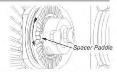
19. Insert the non-slotted driver as shown, making sure the paddle opening in driver (missing extended tooth) is facing out towards you.
