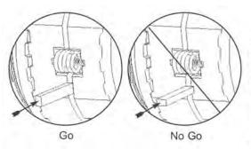
**32.** Check the gap between drivers using check block. The narrow side of the block should fit between the drivers, but the wider side should not fit.
