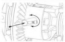
**39.** Using the retaining bolt/roll-pin as a handle, insert the shaft into the differential. Press hard while twisting to pass shaft by springs.
